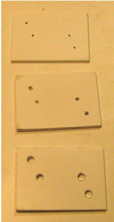
Three stages of LED board manufacture.
