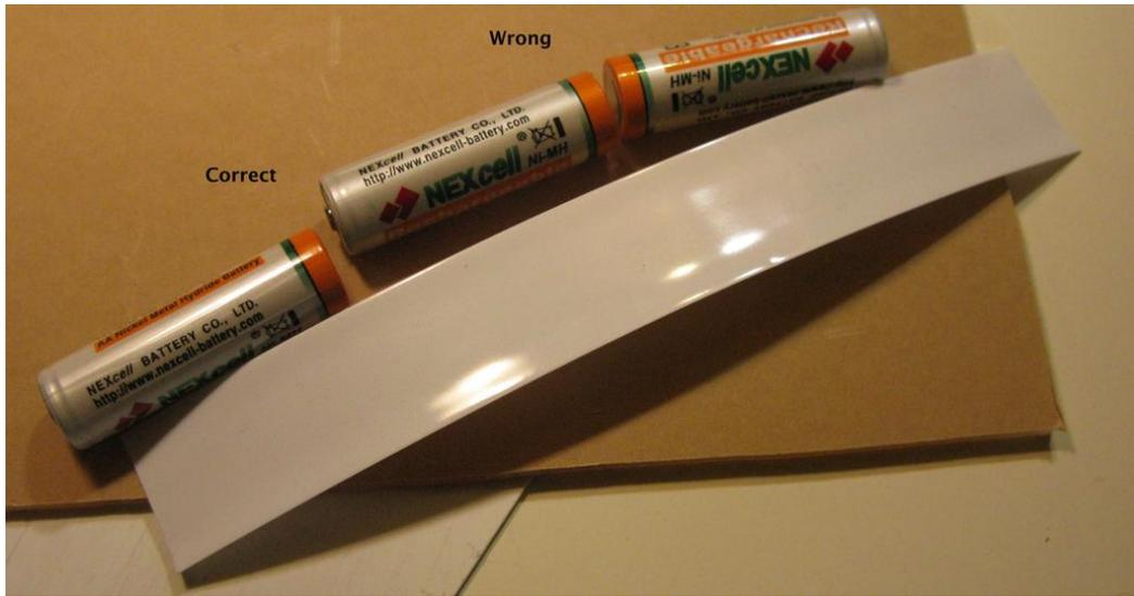
4.2 Gently heat the shrinkfit to hold the batteries firm making sure they stay in contact. Trim off the spare plastic to show the ends of the battery pack. Again check the voltage.
