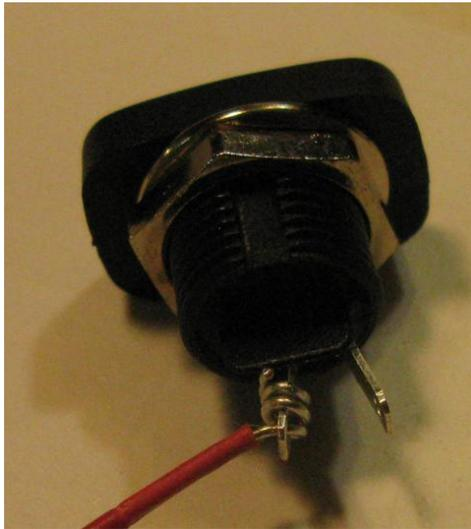
2.4 Cut two pieces of narrow shrinkfit, each 1 inch long and slide them over the wires so that they reach as close as possible to the switch and cover the windings. Gently heat the shrinkfit and it will seal the wires onto the switch.
