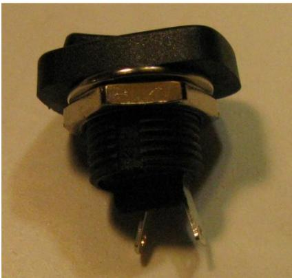
2.3 Feed the long end of one wire through the hole in the end of the switch and then wrap the stripped part of the wire round the switch leg tightly. Use the needle nose pliers to help you make sure it is tight. Then do the same to the other leg.
