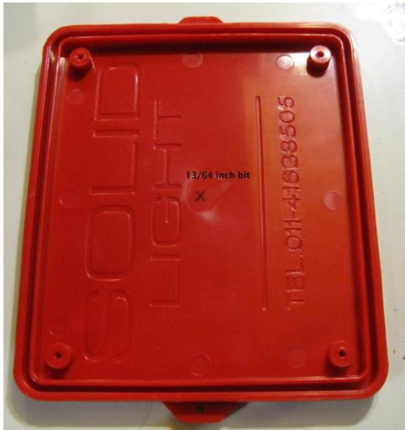
1.2 Use template 1 to mark holes in the short sides of the housing lid. Pass the solar panel leads through the hole in the centre of the lid.
