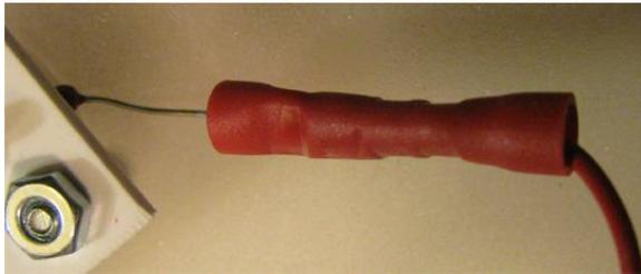
7.3 The solar panel wire needs to be shortened to 10 inches and then the two sides of it stripped apart.
