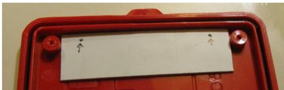
Centre the lid on the solar panel and make sure the sides align as closely as possible. Using a 1/16 inch (or 5/64 inch) bit drill one hole through the lid and the frame of the panel. Do not press to hard when you are drilling through the metal. Use #4 3/8 inch self-tapping screw and fix the lid to the panel at the first corner.
