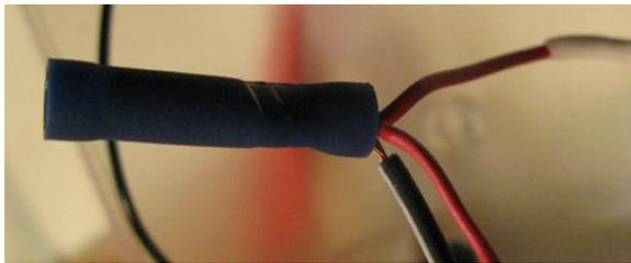
7.4 Take the negative side of the solar panel, the black wire from the LED board and the black battery connector and join them together with a blue connector.
